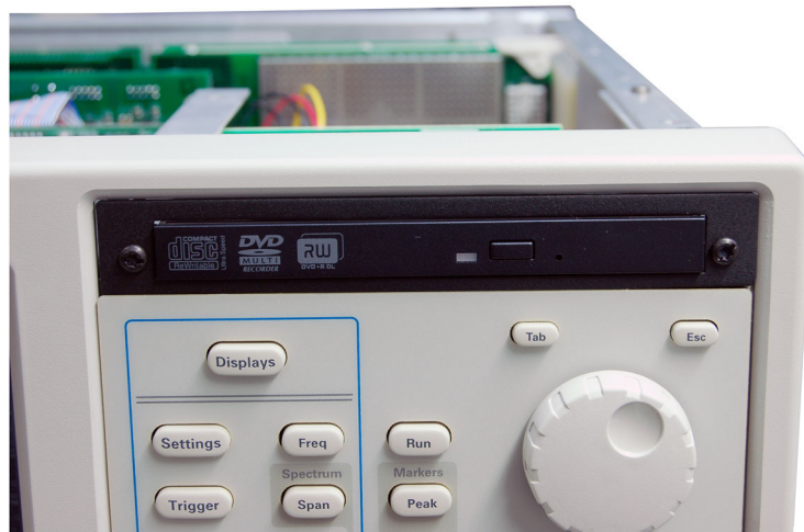
Figure 16: Installed DVD trim ring
